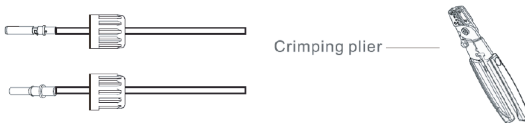
Pic 5.4 Crimp the contact pin to the wire
